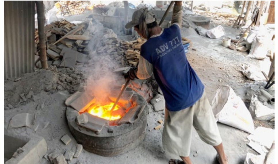
Photo 8: Smelting process using firewood. Photo: Nexus3.
