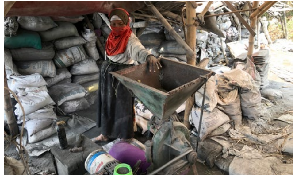
Photo 6: A crusher is used to refine the size of the slags. Photo: Nexus3.
