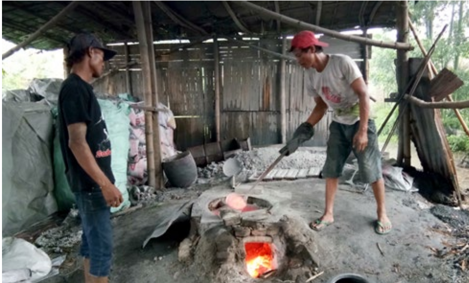
Photo 9: Pouring hot melted aluminum into the cast. Photo: Prigi Arisandi, Ecoton.
