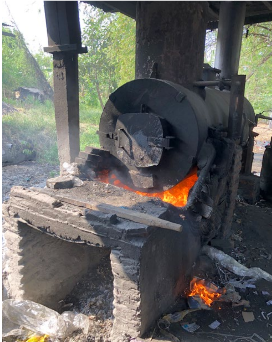
Photo 16: Plastic scraps burned in a simple furnace to create steam. Photo: Nexus3.
