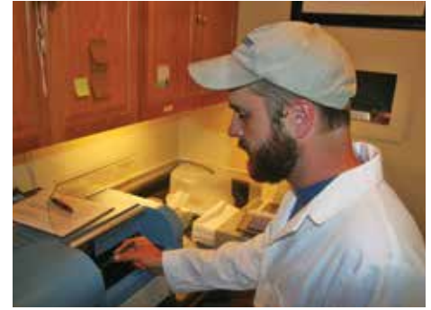
Samples were analyzed on BRI's Milestone DMA 890, using a U.S. EPA-approved method (SW-846 Method 7473).
