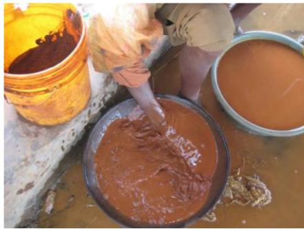
Fig 4. Gold ore amalgamation in ore processing pond
