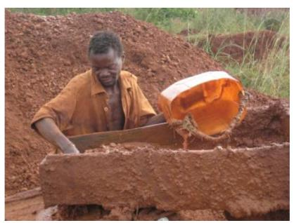
Fig 1. Individual miner re-sluicing tailings
