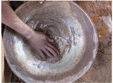
Fig 5. Finalizing gold ore amalgamation on the side of ore processing pond
