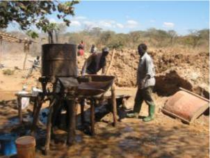
Fig 3. Gold ore sluicing by using constant flow employing the siphon method at Makongolosi mining center, Mbeya Region
