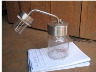
Fig 9. Glass retort that were distributed during Global Mercury project in Lake Victoria zone
