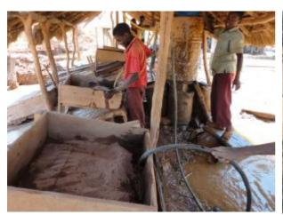
Fig 2. Gold ore sluicing by using constant flow employing the siphon method at Katente mining center, Shinyanga Region
