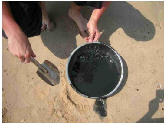
Picture 29: Sediment sampling with a shovel at MTP1-14
