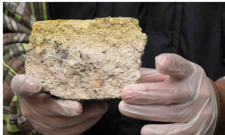
Photo 11.1: POPs pesticides can accumulate at sites of their storage and preparation, as seen in one building in Klatovy, Czech Republic, which was found highly contaminated with DDT and lindane (Dvorská et al., 2007; Møller, Straková, et al., 2020). The photo shows a contaminated part of the wall. Photo: Jindrich Petrlik, Arnika, October 2010.
