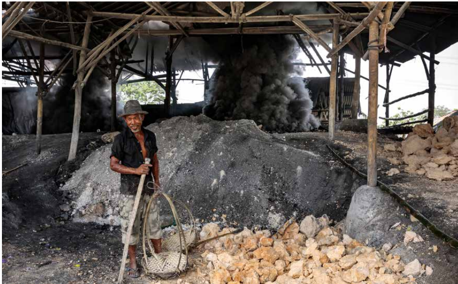
Photo 5.2: Plastic waste is used as fuel in lime kilns in Karawang. Photo: Ondrej Petrlik, Arnika, December 2022.
