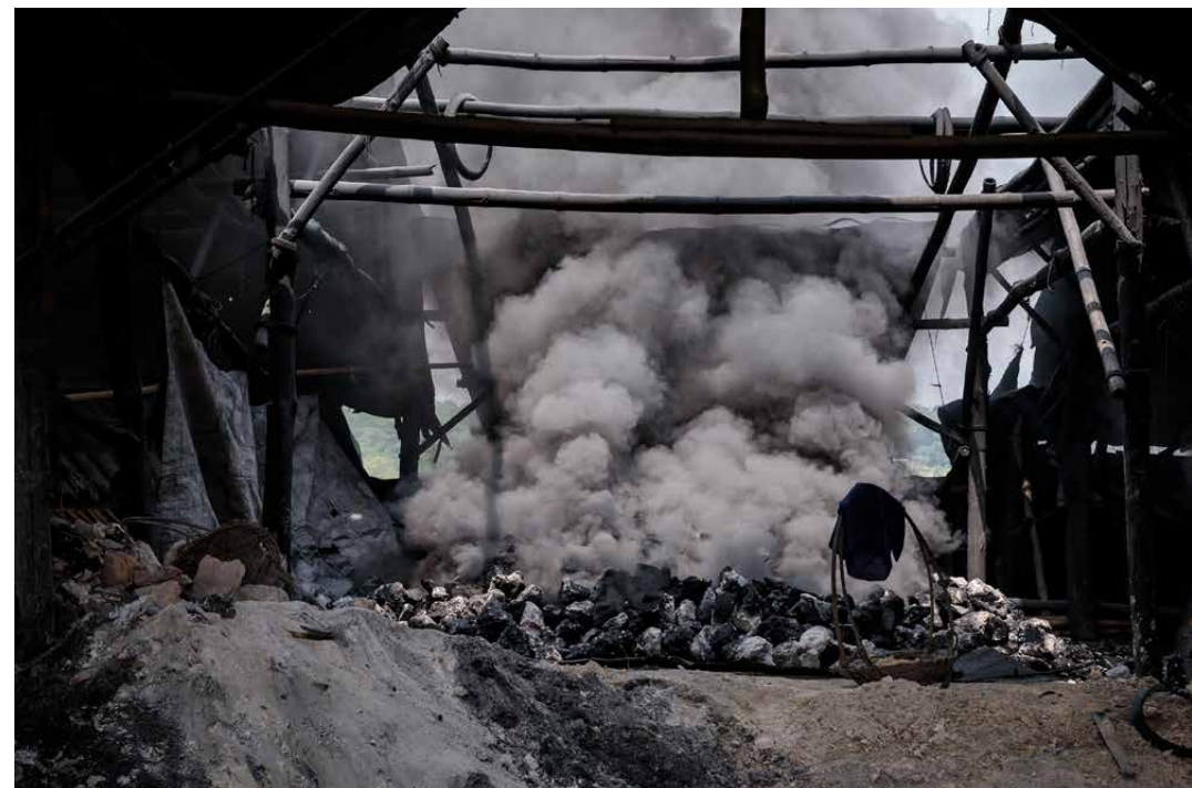
Photo 5.5: Exhaust gases and ash from burning plastic waste in lime kilns in Karawang caused serious POPs contamination of the environment and food chain. Photo: Ondrej Petrlik, Arnika, December 2022.
