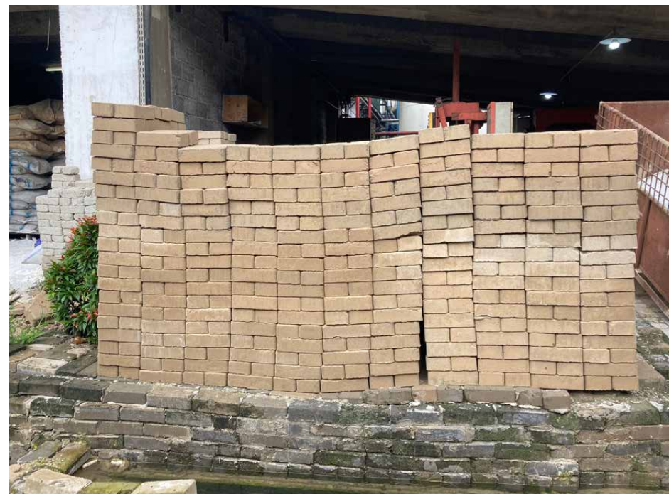
Photo 6.6: Bricks made of fly ash from a waste incinerator, and their use within the area of the facility itself at the bottom. Photos: Jindrich Petrlik and Nikola Jelinek, Arnika, December 2022.
