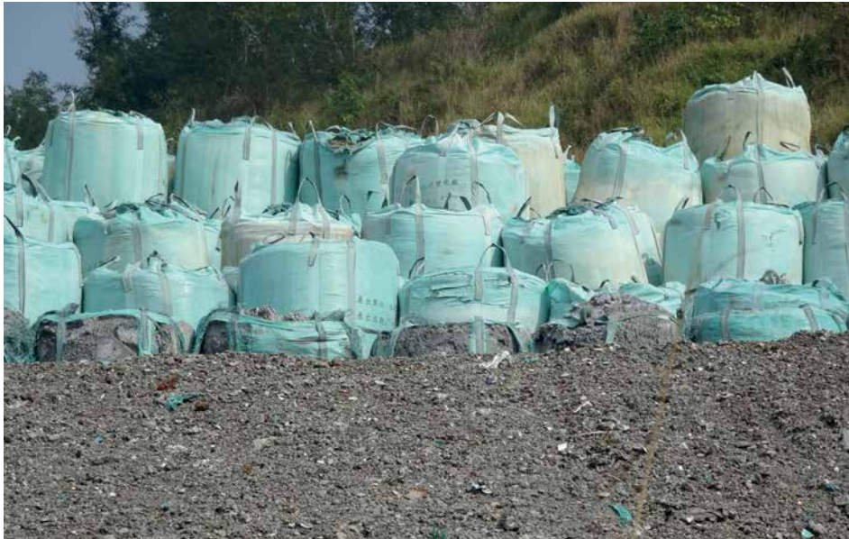
Photo 3.20: This is what solidified fly ashes (mixed with cement) look like at the Yan Chao site in Taiwan (Bell et al., 2023a). Photo: Jindřich Petrlík, Arnika.
