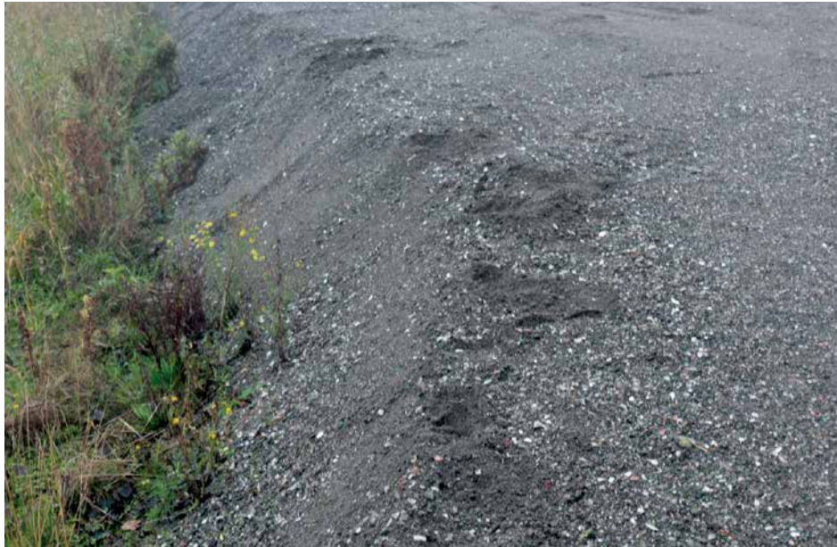
Photo 3.26: The use of bottom ash from municipal waste incinerators in Katwijk aan Zee disregards potential water contamination, as seen in a photograph from November 2021. Photo: Jindřich Petrlík, Arnika.
