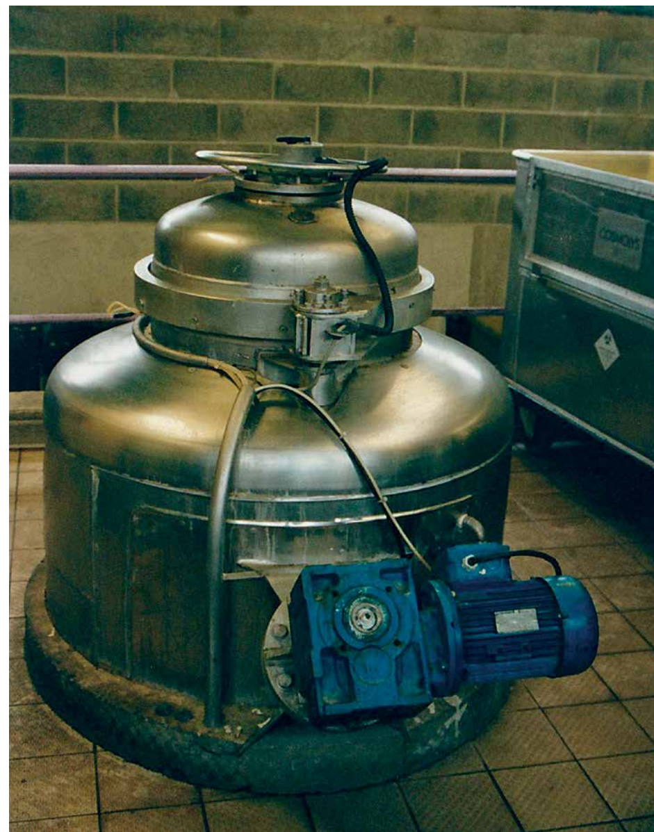
Photo 8.5: Autoclave by the French company Ecodas installed in one of the French hospitals. Photo: Jindřich Petrlík, Arnika.
