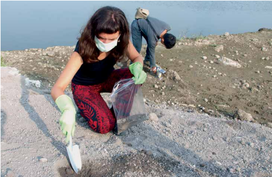
Photo 3.14: Sampling of ash from the Taiwanese incinerators at Anciao Road in 2016 (Bell et al., 2023a). Photo: Jindřich Petrlík, Arnika.
