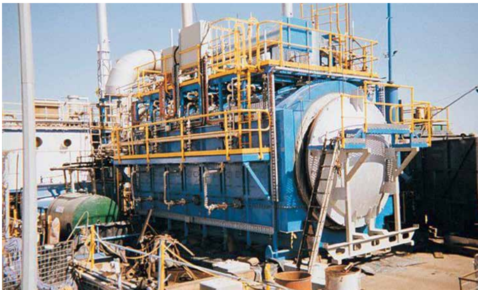
Photo 3.18: Gas-phase chemical reduction (GPCR) technology used in Australia. (Source: Arnold, 2003)
