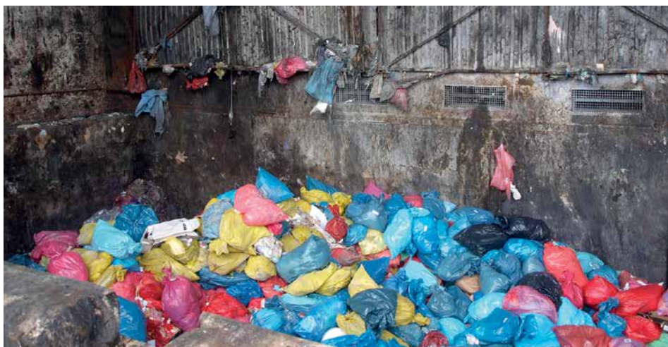
Photo 8.8: Medical wastes in incinerators can be identified by packaging in colored plastic bags. The photo shows medical waste prepared for incineration in the hazardous waste incinerator in Trmice, northern Czech Republic. Photo: Jindřich Petrlík, Arnika.
