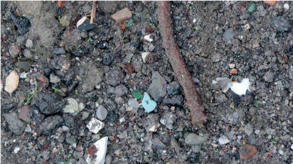
Photo 3.28: The presence of various unburned residues of metal, glass, or even plastic waste indicates that it is ash from waste incineration. Photo: Jindřich Petrlík, Arnika.
