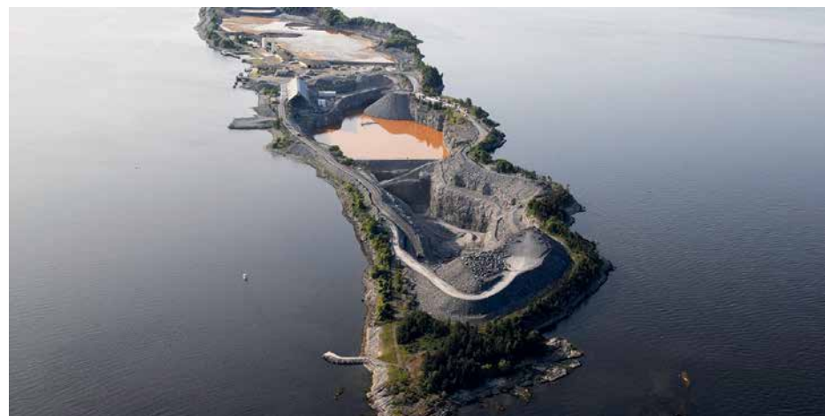
Photo 3.22: Fly ash from extensive Swedish incinerators ends up in an old limestone quarry on the Norwegian island of Langøya in the middle of the sea near Oslo. As noted by the photographer, the island's nature has suffered; the reserve on the eastern coast is slowly dying. (Source: Opie, 2015)
