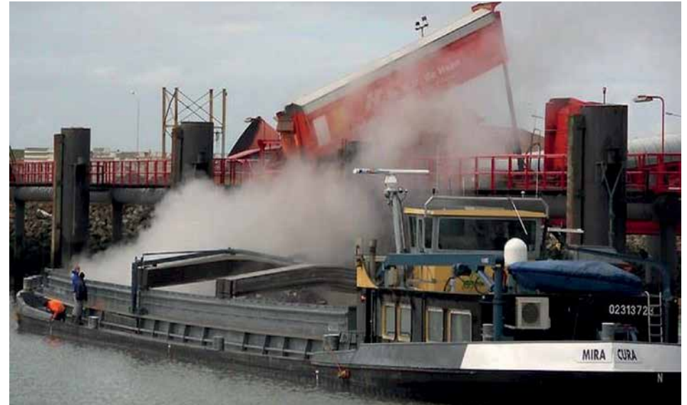
Photo 5.2: Dioxins can spread through fugitive emissions, such as when handling residues from waste incineration, as depicted in this image from Harlingen, the Netherlands, or Photo 4.6 from a hazardous waste incineration plant in Jihlava, where noticeable dust leakage occurred during fly ash handling. Photo: ToxicoWatch. (Source: Arkenbout & Bouman, 2018).
