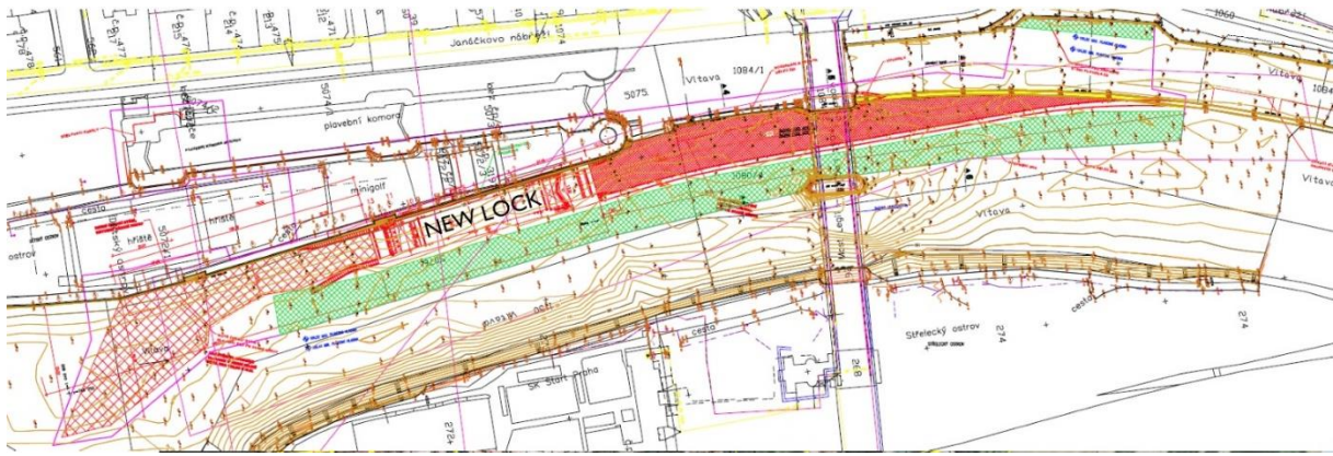
Fig 7 Plan of the proposed second Smíchov Lock.
