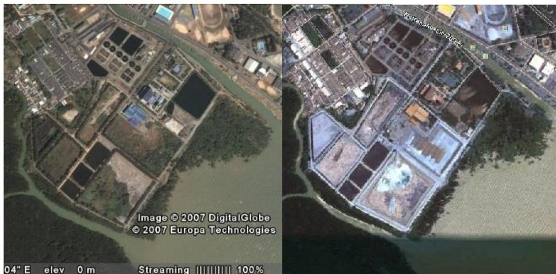
**Picture 2:** From the comparison between photomap from 2007 (left side) and 2010 (right side) is clear, that land use has changed around waste incinerator in Phuket. Large grey area at south east edge of the incinerator was area with fly ash dumping in 2007.
