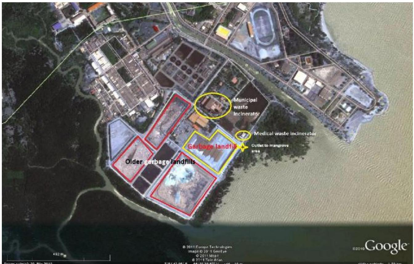
**Picture 1:** Map of the Phuket waste landfill/waste incinerator complex with description of its parts. Google Earth map was used as basis at this picture.
